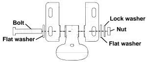
Assemble transducer and bracket.
